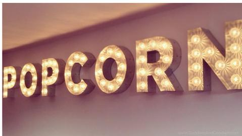
**Individual Exposed Bulb:** Individual exposed bulbs can be used to highlight particular elements of sign copy, or to animate a sign to make it more eye-catching. Individual bulbs may project from a flat sign or embedded within a Projected sign, but the light source is always visible from the public right-of-way.
