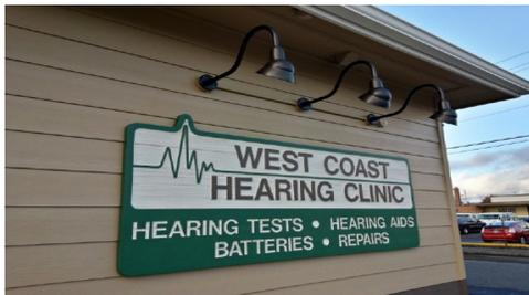
**External:** Signage can be illuminated with spotlights aimed upward at copy, or hooded lamps that shine downward upon it. Each light source is fully independent of the sign itself.
