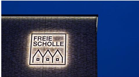
**Halo Lighting:** Opaque sign copy can be illuminated by diffuse light from sources mounted behind copy, creating a ‘halo’ effect around the copy elements. Light sources should not be visible from the public right-of-way.
