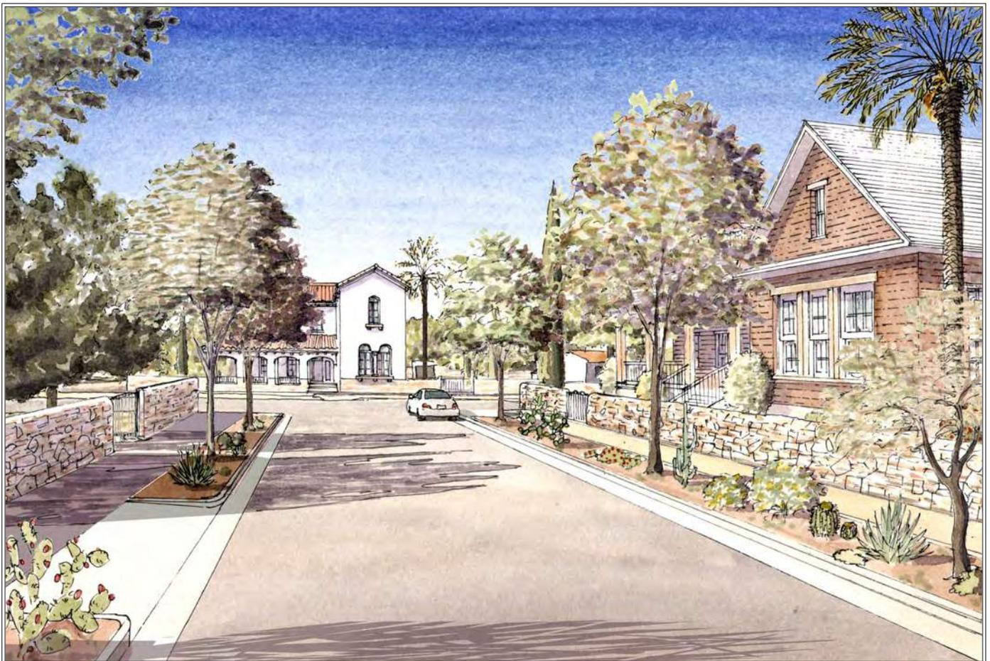
STEP 4: Redesign of the roadway should be undertaken to narrow the curb-to-curb dimension, thereby increasing the perception of visual friction and discouraging speeding. Planting strips should be landscaped with desert-appropriate species and groundcover.
