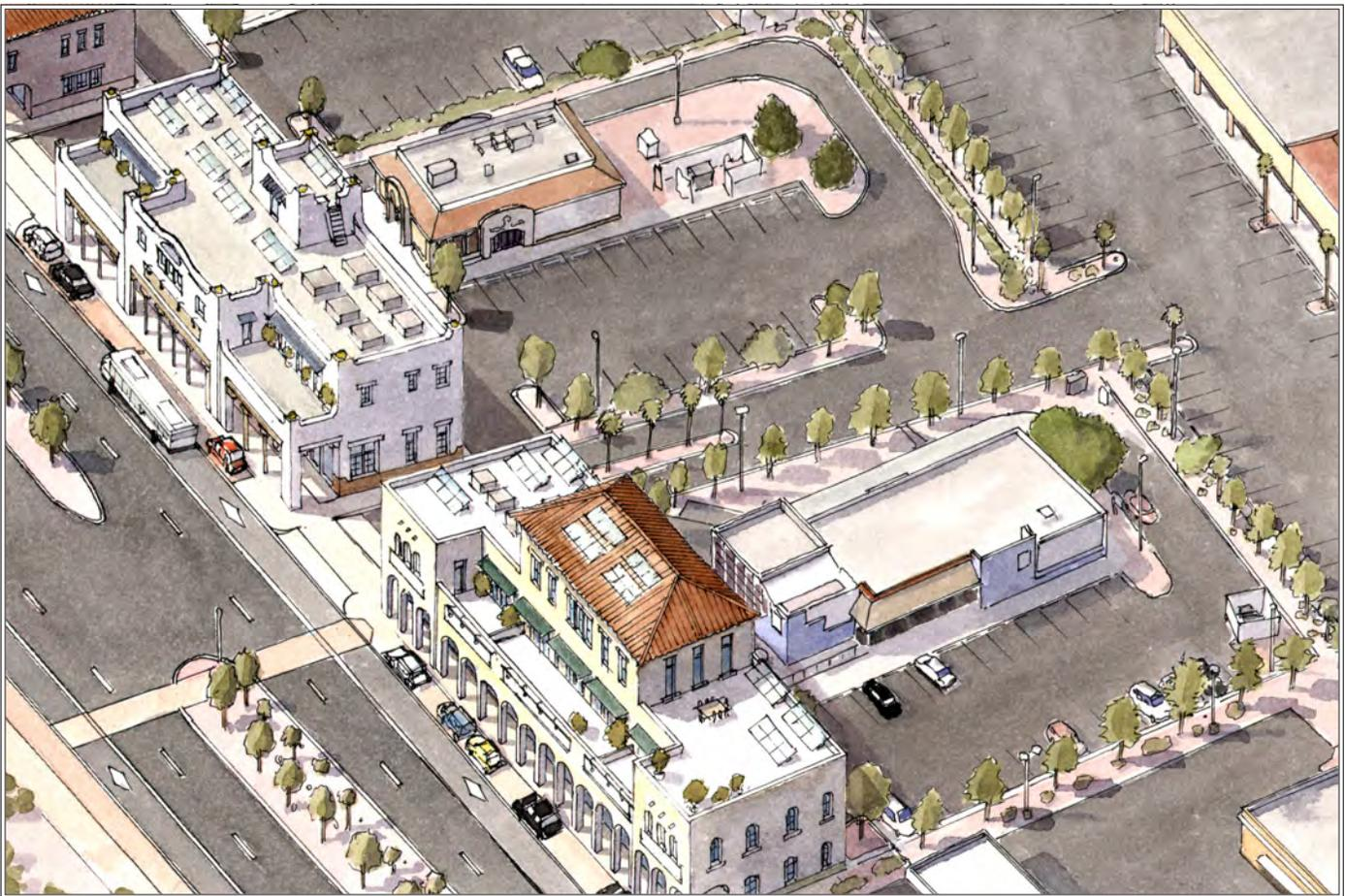
Step 2: Infill buildings provide a continuous street wall along Montana Avenue and colonnades shade the sidewalk. Driveways and intersecting streets should have speed tables to make the sidewalk appear continuous. Roof terraces can have private outdoor space for offices or apartments and photovoltaic panels on the roof can reduce reliance on the electrical grid.
