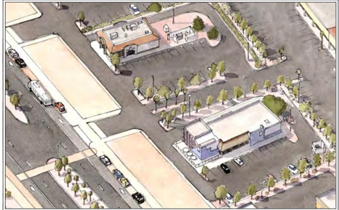
Step 1: The main arterial is reconfigured; the outermost lanes re-striped to accommodate buses. On-street parking is added, sidewalks are made more continuous, and crosswalks are added. Parking lots are reconfigured to allow for building pads at the fronts of the lots, while the rear portions of the lots are planted with shade trees; drive-thrus remain.
