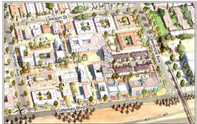
CPTED Solutions, Step 3: Desert-adapted trees and plants are installed on existing and proposed planting strips and swales. They are spaced wide enough and staggered in order to maintain surveillance "line of sight" across public spaces.
