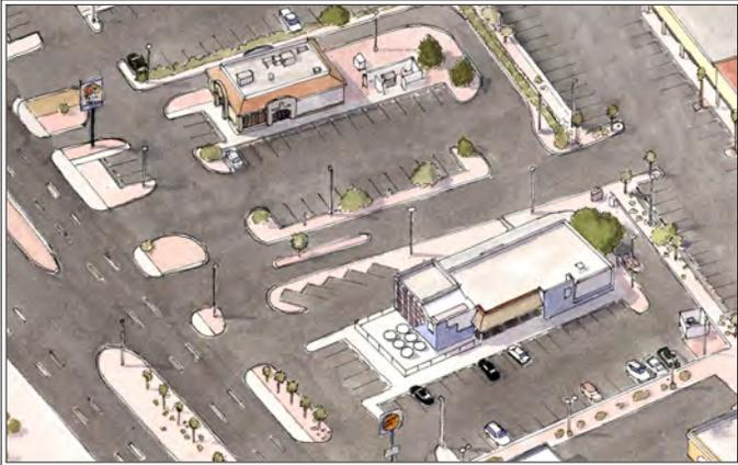
Existing Conditions: Currently, there are too few crosswalks between Bassett Place Mall and the opposite side of the street. The sidewalks are discontinuous due to the number of curb cuts and rather than forming a street wall, buildings poke out of parking lots.
