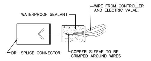
THREE STEP OPERATION DRI-SPLICE CONNECTOR ONLY. FILL WITH SEALANT SUFFICIENT TO SEAP WHEN ASSEMBLED.
