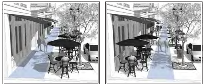
Five feet of pedestrian clearance is required. Wide sidewalks can provide a greater length for greater pedestrian comfort.
