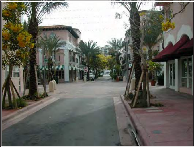
An example of a curbless intersection that features bollards and a high degree of spatial enclosure, resulting in slow driving speeds.
