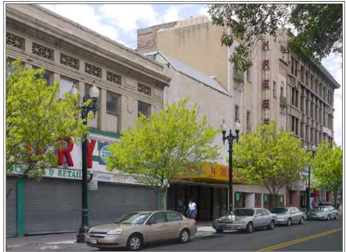
STEP 1: Pedestrian Infrastructure Add regularly planted shade trees along the sidewalk and add pedestrian-scaled lighting to enhance the safety and character of Downtown. Pedestrian-scaled lighting should be designed to also create safe conditions for drivers. The addition of on-street parking will also create a calmer pedestrian environment and make shopping Downtown more convenient.
