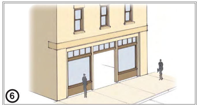
⑥ Cased windows sit atop knee-height bulkheads
