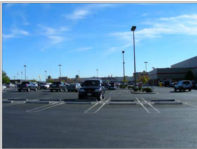
Sun-baked, mostly treeless asphalt surface parking lots, along with low albedo surfaces such as dark roofs, contribute to the urban heat island effect. This leads to higher cooling bills and greater discomfort for pedestrians on hot days.
