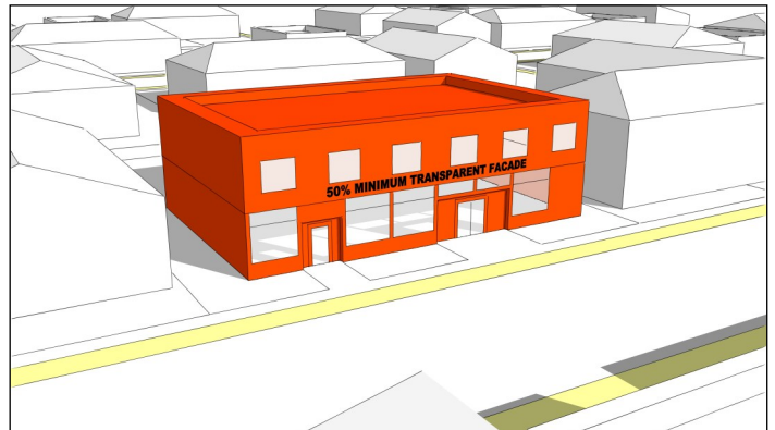
To calculate percentage of transparent surfaces, determine the total area of the first floor façade. Any transparent glass surfaces within that total area can be counted toward the requirement.
