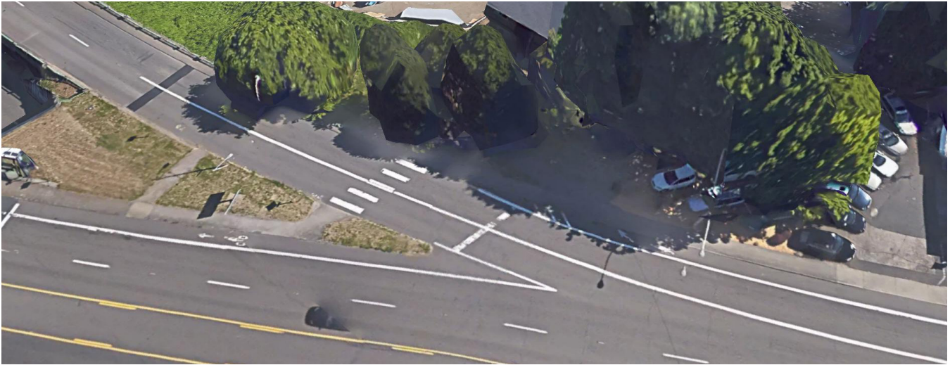
Figure C15. In constrained conditions, bicyclists may exit onto the sidewalk and complete the maneuver with pedestrians in the crosswalk, as in this example from Portland, OR. Bicyclists may choose to exit the bike lane and make a vehicular style transition if they prefer.
