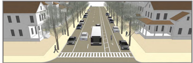
Step 2: Another intervention in the design of East Yandell envisions the installation of a buffered bike lane that would be achieved by eliminating one travel lane.
