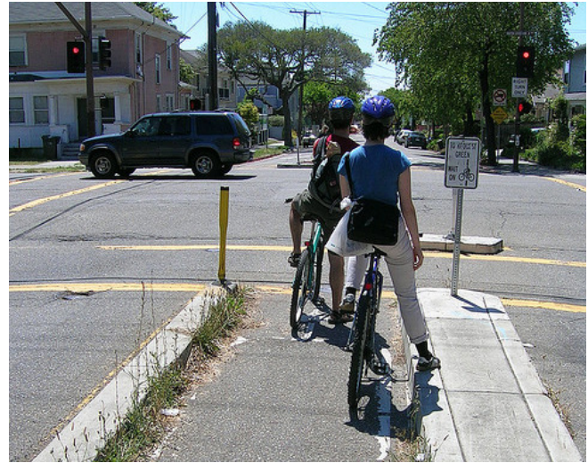
Figure C12. A bicycle detection system triggers a change in the traffic signal when a bicycle is detected.
