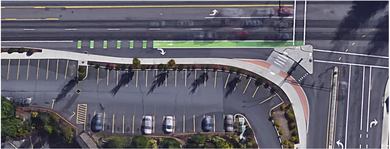
Figure C13. This example uses a raised, mountable apron at the corner to define a tight corner radius for passenger cars.
