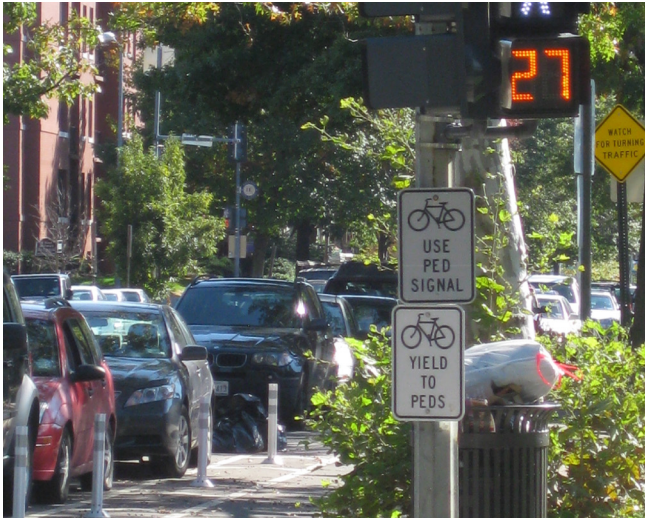
Figure C11. A bicycle signal head at a signalized crossing creates a protected phase for cyclists to safely navigate an intersection.
