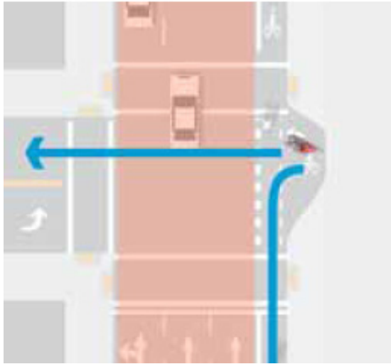
Figure C2. This MUTCD compliant design curves a jughandle out of the sidewalk to provide space for waiting bicyclists.
