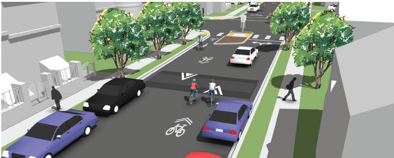
Figure C22. Bicycle boulevards incorporate signs, pavement markings, and traffic calming measures to discourage through trips by motor vehicles while accommodating local access.
